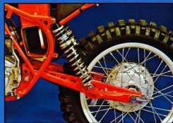
The rear shock mounting allows 240 mm of rear wheel travel.
