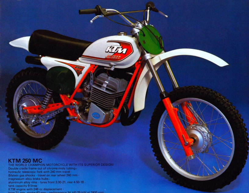
Light-weight Moto Cross frame made of chrome-moly tubing.
