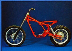
Light-weight Moto Cross frame made of chrome-moly tubing.
