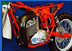
New lightweight airfilter box with larger filter unit.
