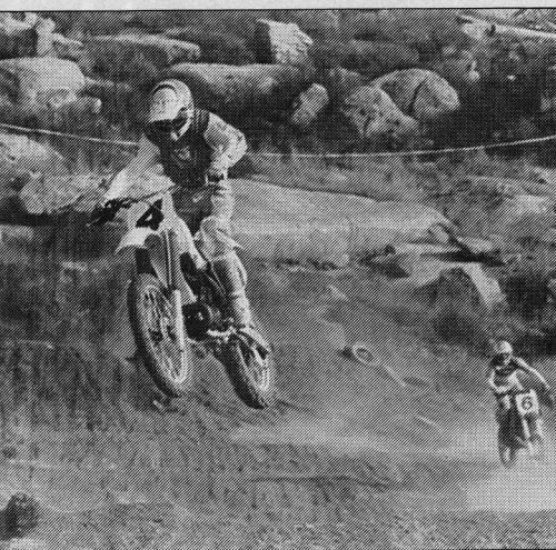
Because the YZ's rear shock is so overdamped on the initial travel, it wants to stand up in midturn and kick on square-edged holes. On the other hand, it likes to go straight and makes a good desert bike.
