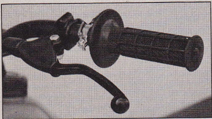
Levers are made from forged aluminum, are easy to reach, have double bolt pedestals that are easy to replace. Grips are some of the best ever put on a production bike and have safety wire grooves.
