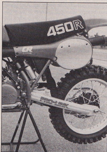
Pro-Link swing arm is made from extruded aluminum. Conical rear hub has large diameter spokes. Shock reservoir is aluminum and uses a piston to separate the nitrogen and oil. Seat is thick and comfortable.
