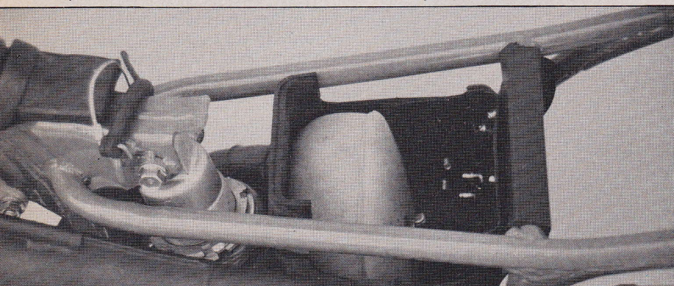
Spring preload is adjusted by turning the ring at the top of the shock body. Airbox is good design that has a splash dam at front and rear, air inlet at each side. Filter is oiled foam.
