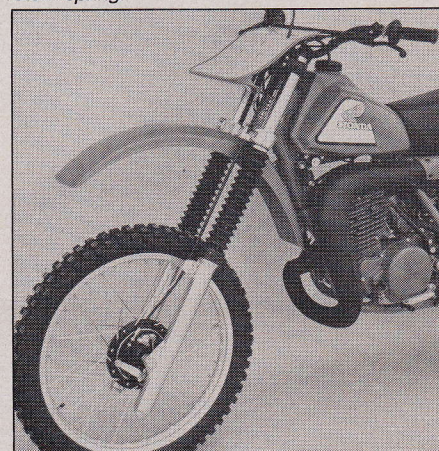
Double leading shoe front brake furnishes strong, progressive stops with no suddenness. Brake cable clamp is extra wide so cable doesn't flex into tire when landing from high jumps. KYB forks have 41mm stanchion tubes and long lower legs for good engagement. Normal damper rods, not cartridges, do the damping. Fork boots have flat inners for tire clearance. Headpipe extends below frame several inches. Gas tank is plastic.
