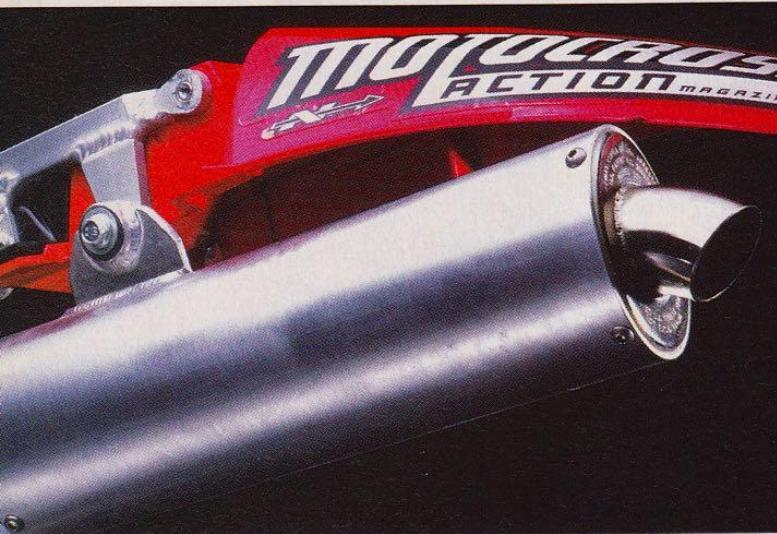
**Misfire:** MXA's Cannondale came with a Big Gun exhaust system, but Cannondale plans to switch to FMF pipes. Space confines doom any exhaust pipe to mid-and-up power only.
