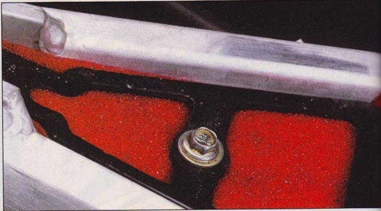
**Back up:** In our opinion, the air filter behind the front number plate doesn't flow much air. The sandwich filter, located under the gas tank, is the main source of air for the engine.
