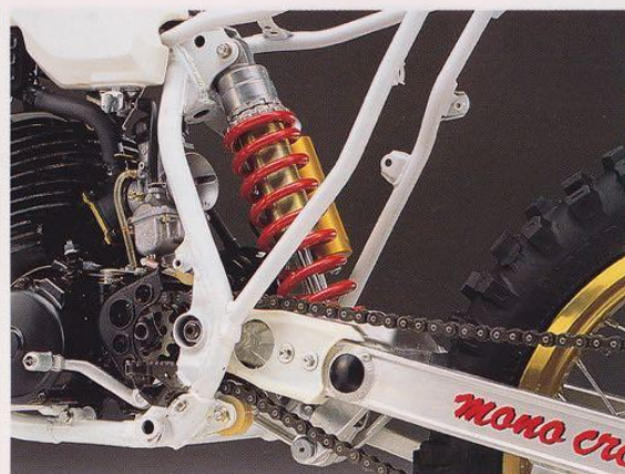
New rear shock and remote reservoir provides better rebound and damping.
