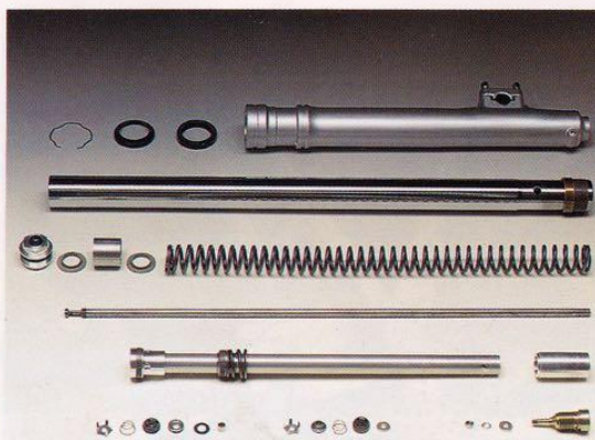
New cartridge forks for more efficient compression and rebound damping.
