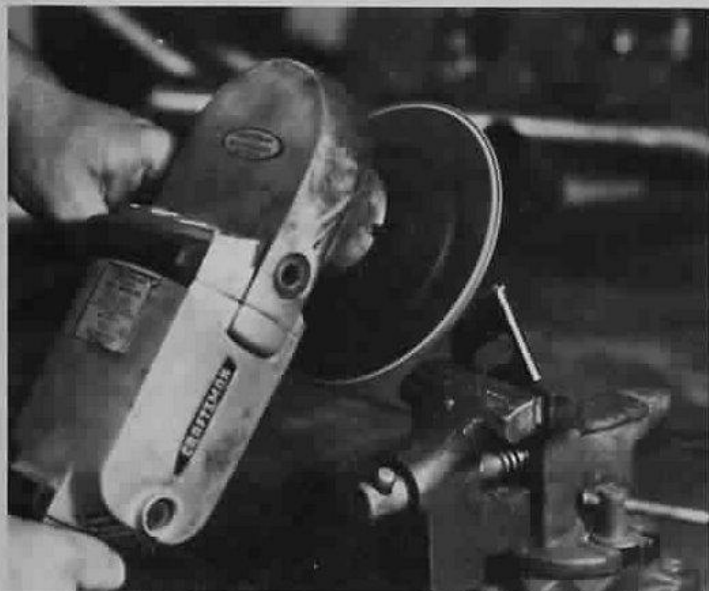
7. Place the cut off tab in a vise and grind the leading (cut) edge to a "V". Grind about 1½ inches back on the bottom of the axle mounting tab. The extension piece will weld on here.
