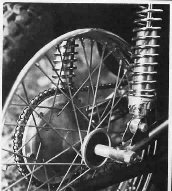
Ceriani suspension front and rear make for a spectacular handling machine. Conical hubs are cast magnesium alloy and keep unsprung weight down to an absolute minimum.
