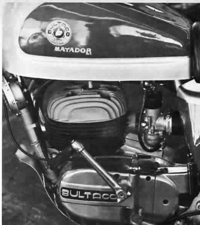
Finish of the Matador was quite good. Carburetion is by 32mm Amal. Skid plate is effectively designed.
