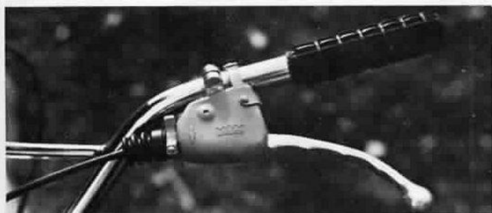
Outstanding feature of the Micro-Metisse is the use of Magura controls and levers. Rubber covers over pivot points keep the muck out of the moving surfaces. Large plastic knobs allow easy adjustment of cable tension. Levers will bend back.
