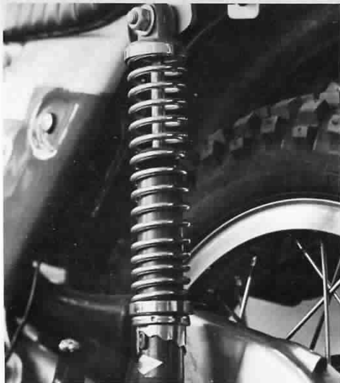
Betor shocks could be bottomed coming down after a jump but generally provided smooth, stable ride even in the rough.
