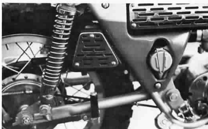
The muffler attaches to the exhaust with a rubber hose and two bolts. Even without the muffler, the Matador has a subdued, mellow sound. Tool kit is contained in inset canister.
