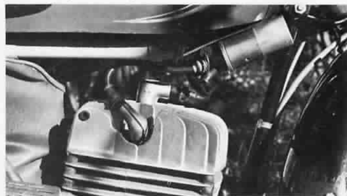
Engine features dual ignition, a nice feature on any bike and uncommon on an enduro machine. Finning is more than adequate as engine was never too hot to the touch even after hard running.
