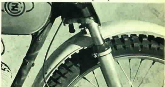
Hard braking action will almost bottom out even the finest front suspension made today. This graphically illustrates just how much weight is on the front end.
