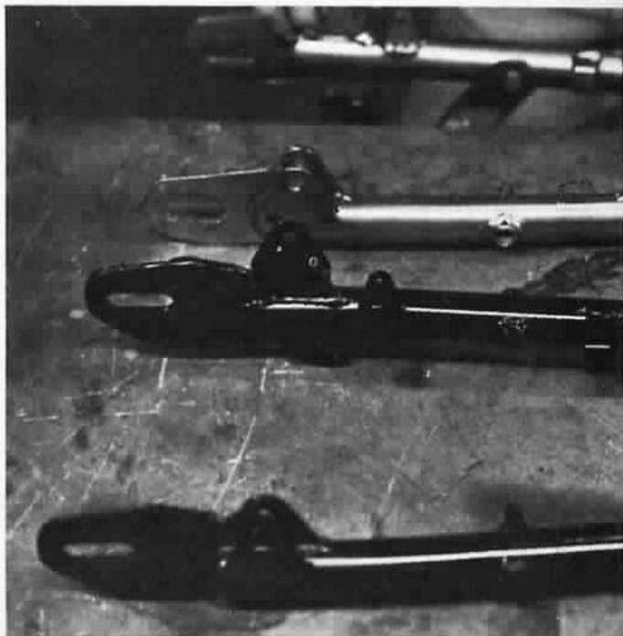
16. A comparison of the stock and extended swingarms for the AT-1. It's not THAT much different but the resulting handling is!
