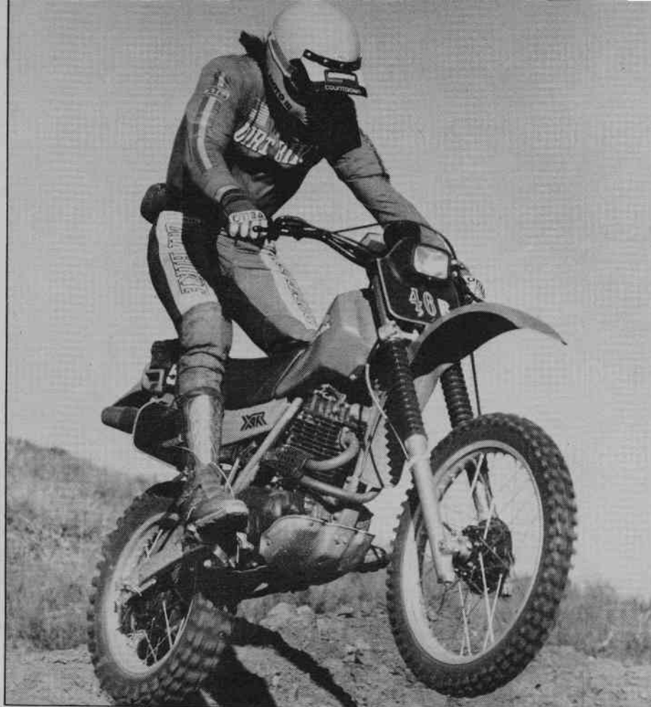
Chain adjustment was a snap; snail adjusters simplified the process. Rear wheel was quick-disconnect. Six-ply IRC Vulcanduro was a real rock eater but didn't hook up well in deep sand. We eventually used a Terraflex 4.10 x 17 close-knob for improved traction.
