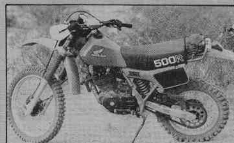
Here's what our bike looked like all set up for the Tough E'Nuff Enduro. A White Bros. pipe, lots of tools and a Countdown Combo clock were used. Yamaha hand protectors helped keep the heavy brush from whacking knuckles. At the end of the 100-miler, the Honda was running just fine.
