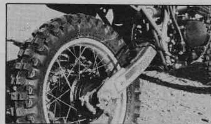
Chain adjustment was a snap; snail adjusters simplified the process. Rear wheel was quick-disconnect. Six-ply IRC Vulcanduro was a real rock eater but didn't hook up well in deep sand. We eventually used a Terraflex 4.10 x 17 close-knob for improved traction.
