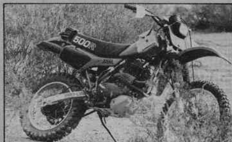
Here's what our bike looked like all set up for the Tough E'Nuff Enduro. A White Bros. pipe, lots of tools and a Countdown Combo clock were used. Yamaha hand protectors helped keep the heavy brush from whacking knuckles. At the end of the 100-miler, the Honda was running just fine.
