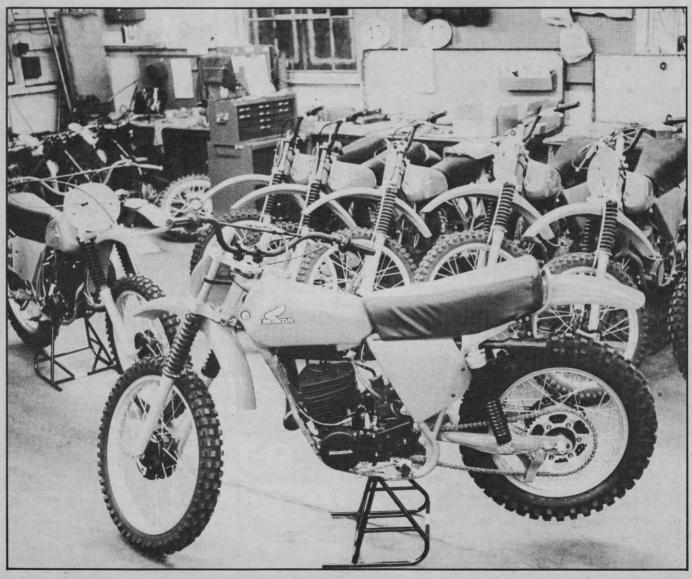
Honda experienced early frame breakage but solved the problem by using better materials and a few well-placed struts. Different flywheel weights are used to suit rider preference.
