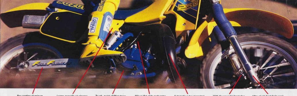
Box-section aluminum swingarm is lightweight and flex-resistant for great stability. Larger-capacity air cleaner lets the engine breathe more easily for more power. Tough, quick-shifting transmission (6-speed on RM125; 5-speed on RM250).
