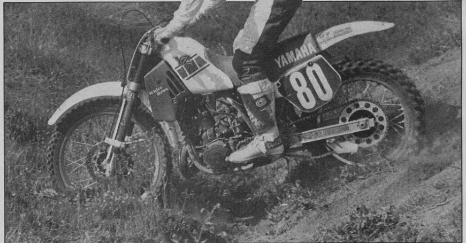
Under heavy loads, the White Powers track straight. With the sliders on top and the legs underneath, the binding, twisting and flexing forces are better contained.
