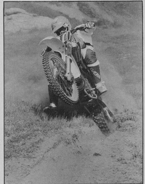
Under heavy loads, the White Powers track straight. With the sliders on top and the legs underneath, the binding, twisting and flexing forces are better contained.
