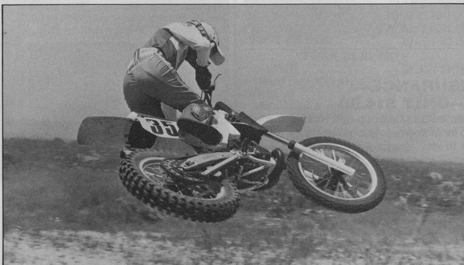
The slim seat and tank give the rider a good fit and make midair acrobatics fun. The antiquated 40mm Swedish-built forks don't make coming in for a landing half as much fun. Stiction, lack of rebound and a tendency to bottom plague the Hooska forks.
