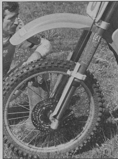
Under heavy loads, the White Powers track straight. With the sliders on top and the legs underneath, the binding, twisting and flexing forces are better contained.
