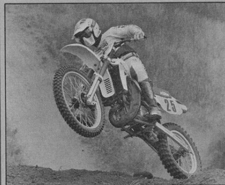
Rock me gently: KTM has a good-handling bike, courtesy of its rigid and ultra-fine forks. Lack of rear shock rebound damping and a fragile pipe hamper its overall rating.
