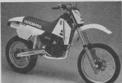
**Husqvarna 510TX Cross Country • \$4995:** Fans of Husky thumpers will appreciate the '88 upgrades to this desert devil. The four-stroke, SOHC, four-valve single-cylinder engine now rides in a new frame taken from the two-stroke line. There are also entirely new body pieces, including tank, fenders, seat, etc., acquired from the same source. The ignition system has been improved, as have the swingarm and rear suspension linkage.
