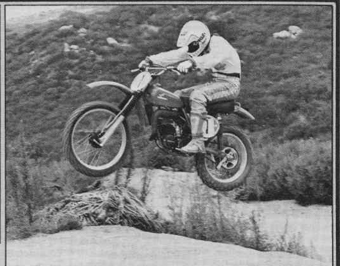
With seven inches of suspension travel on the RC, Marty wasn't anxious to practice any doubles. Both Smith and Micky Dymond thought the 1975 bike made good power but was held back by the archaic suspenders.
