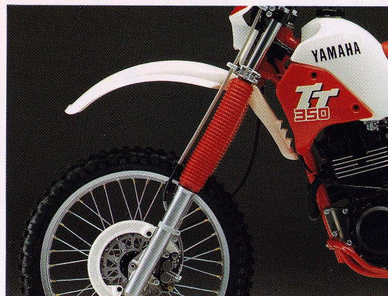
Beefy 41mm front forks on the TT350 resist flex for excellent stability.
