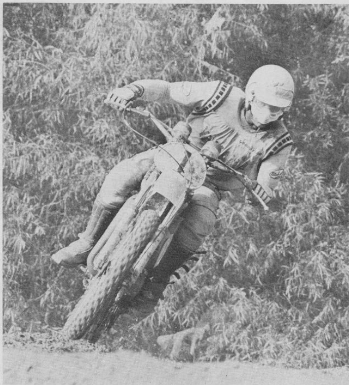
Those aren't dual speedos on Weinert's bike, they're Kayaba (Red Wing) air/gas reservoirs.
