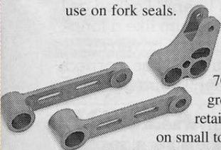
**Suspension Link** The linkage is machined from 7075 T-6 Billet Aluminum, anodized in 'works' grey and is incredibly strong. The suspension link retains stock ride height while increasing plushness on small to medium hits. (Available for '93-'94 YZ125-250 & WR250—\$247)
