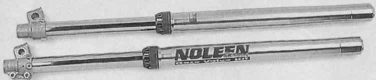
**Fork Fix** Install our famous Works Base Valve Kit (\$89.95) yourself or send us your forks. Our complete Fork Fix features the Works Base Valve Kit, Noleen O-1 Fork Oil, blueprinting and polishing of the cartridge rod, and custom valving tuned to your exact weight and riding ability. (For all makes—\$159.95)
