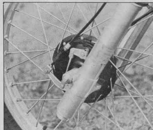
Double-leading shoe front brake is an excellent stopper. After a brief adjustment, you learn to love it.
