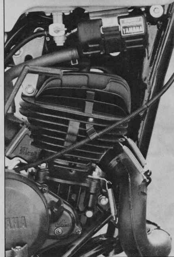
Air-cooled engine has a boost bottle to improve low-rpm response.
