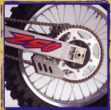
► All-new aluminum swingarm now measures a massive 80 x 36.5 mm for the box-section arms and 18 mm longer for incredibly stiff torsional rigidity and less flex through the gnarliest washboards. The result? Faster acceleration. Straighter tracking. Improved traction. Quicker starts.
