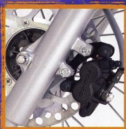
► Just like its big brother KX100, the KX80 comes with a new powerful, twin-piston front brake caliper,
