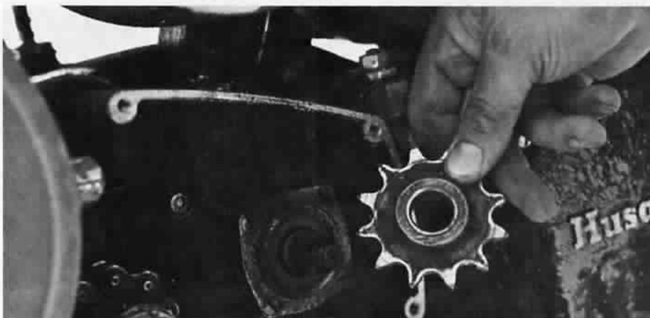
. . . taper fit was not up to the job . . .
