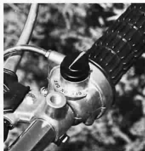
Kaw's Honda-type kill switch will play tricks in heavy brush.
