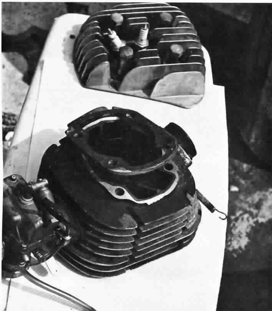
MX cylinder (or ported Enduro cylinder) and Enduro head will do the trick. Use a 32mm carb.
