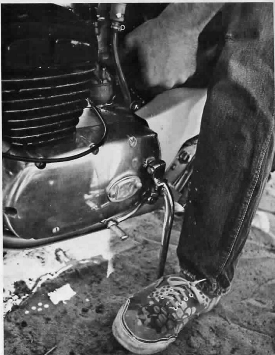
New Amal concentric is vastly improved, but still tinkles on rider.
