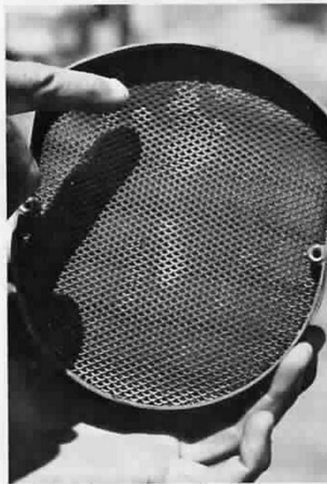
Dirt collects at top of air cleaner. Sealing is needed.
