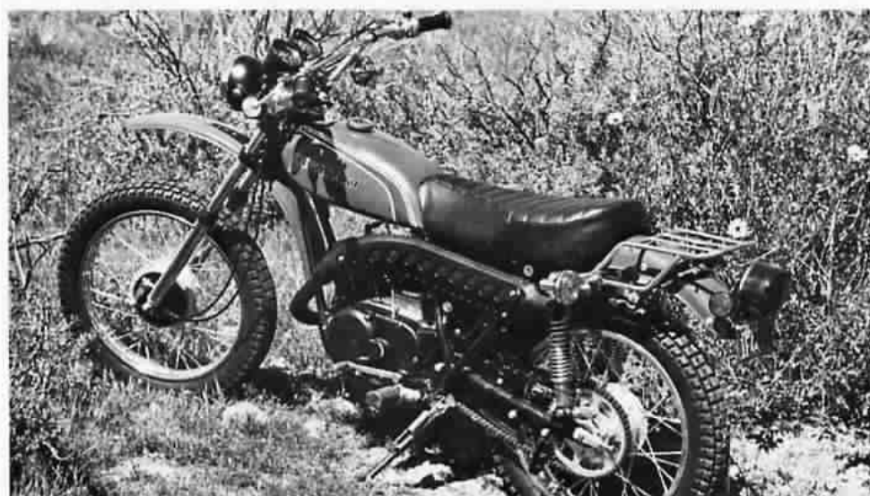
Kaw's Honda-type kill switch will play tricks in heavy brush.
