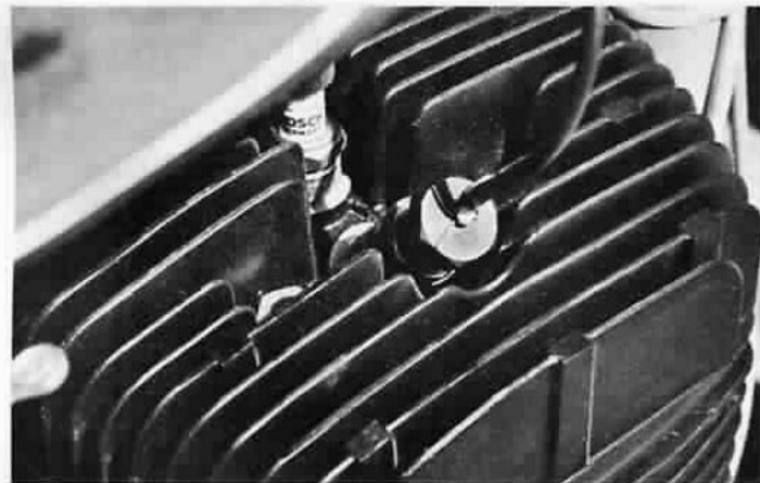
Most modern two-strokes come with an extra compression release/spark plug hole.
