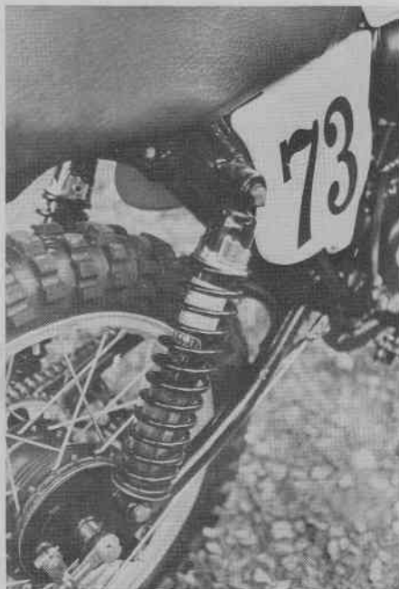
Gas pressure Kayaba laydown shocks work well for a while. Spring rates wither with time.
