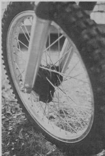
Spokes, both front and rear assemblies, never came loose, a rarity among test bikes. Forks kept the wheel on the ground up to a point. Pitching it at speed over bumps would cause loss of contact and a wash.
