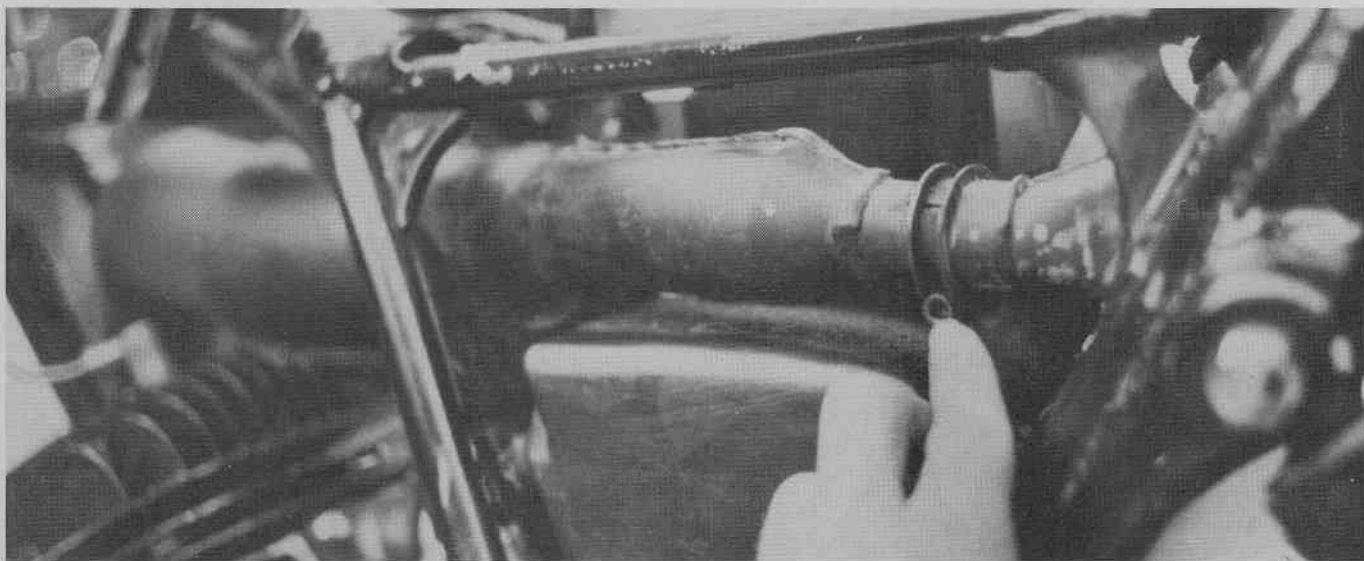
Pipe disconnects easily at this point for quick access to the cylinder. The whole bike is the most easily serviced of any we've tested.
