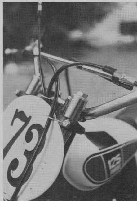
Fork position is adjustable over a two-inch span, cables are heavy-duty and smooth working. Brake cable is well guided and doesn't hang up on the fork tube.
