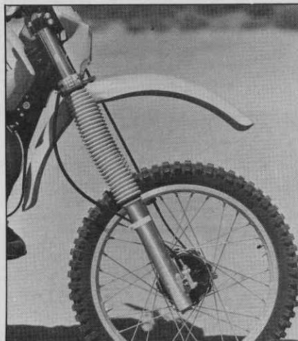
Raising the fork tubes 10mm in the triple clamps helps the front end get a better grip. Fork action is excellent.
