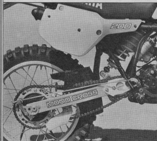
The IT Monocross rear handles suspension chores well at low and medium speeds, but falls short of perfect when the bike is pushed hard.
