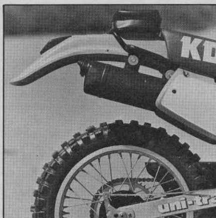
It's quiet and it's heavy: The Kawasaki's massive silencer/spark arrester weighs in at five pounds, nine ounces. Replacing this unit with an aluminum accessory will eliminate about three pounds.
