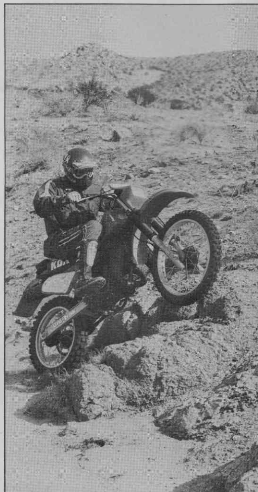
The stock Dunlop K-890 tires work best on dry terrain. In sticky situations they tend to pack up with mud.
