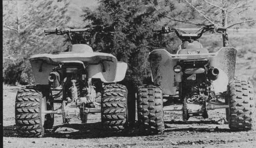
Rear travel on the Suzuki (left) is measured at 8.7" of travel and the Honda (right) is 7.9". As you can see, the QuadRacer is 1" narrower than the FourTrax, which plays a big role in woods riding. Chain maintenance is also easier on the FourTrax. □
